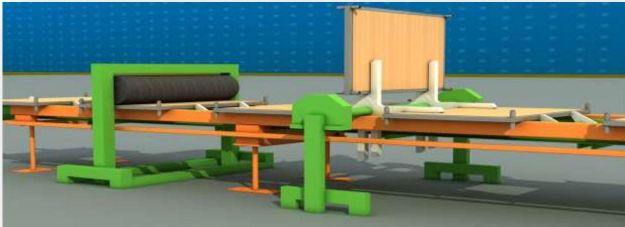
PROVIDES THAT THE PALLETS ARE TRANSFERRED TO THE PRESSING STATION AFTER REVERSING TO USE BOTH SIDES EQUALLY. DRIVEN BY 1,5 kw DRIVE CONTROLLED REDUCER.
