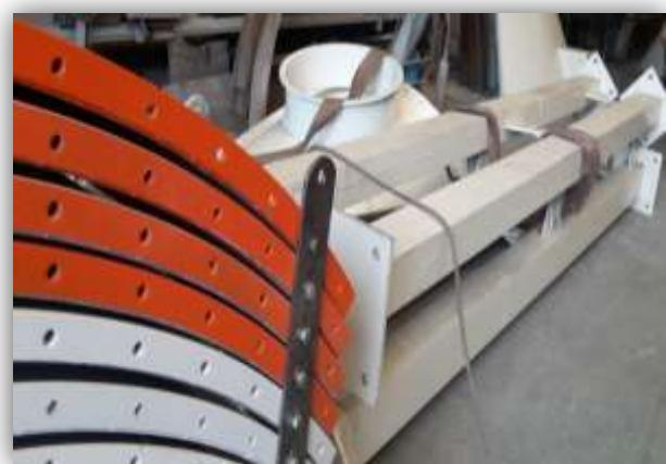
**FOR EASY SHIPMENT; OPTIONAL THE SILO CAN BE MANUFACTURED AS DEMOUNTED ( BOLTED )**
