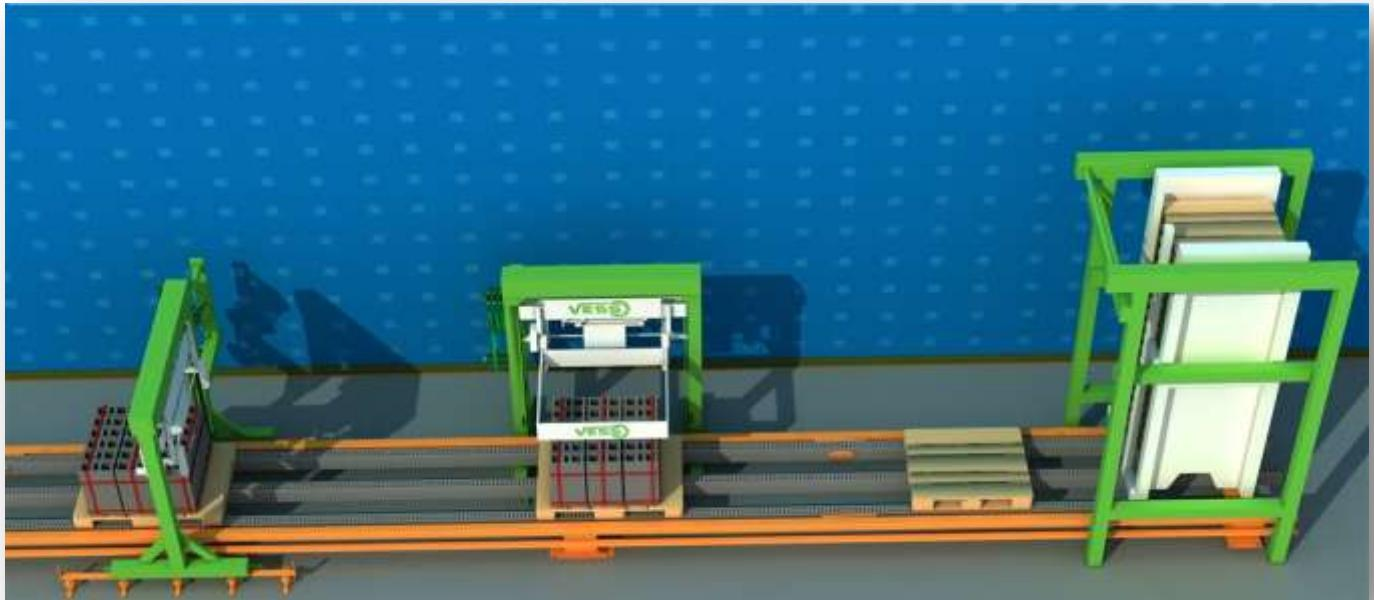
SEPARATE THE PALLETS NEEDED FOR SHIPPING ONE BY ONE AND SEND TO THE PACKAGING STATION.
