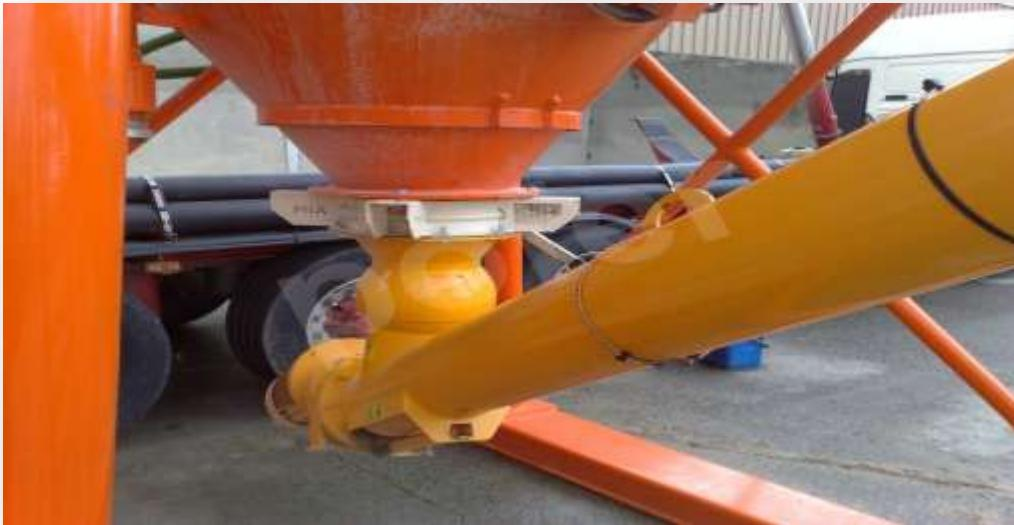
TAKES THE NEEDED CEMENT FOR MORTAR FROM THE SILO TO FEED THE WEIGHING CONVEYOR . WAM BRAND. 8'( $\varnothing 219$  mm ) MOTOR POWER IS 9,2 Kw. SILO CONNECTION POINT IS MOVABLE.
