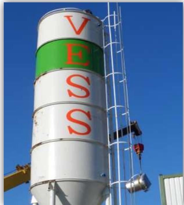
CEMENT STORAGE EQUIPMENT. BESIDES ARE WALKING STAIRS FOR EMERGENCIES. THE CAPACITY IS 75 TON AND REPLACEABLE CARTRIDGE FILTER IS PROVIDED. THERE IS ALSO 2 PIECES LEVEL MEASURING CENSOR PROVIDED AND SAFETY VALVE TO PREVENT OVERFILLING. TO DISCHARGE THE SILO INTO THE CEMENT FEEDING SCREW THERE IS A WAM BRAND VALVE. MANUFACTURED AS STEEL CONSTRUCTION USING 5 /6 mm. SHEET METAL.
