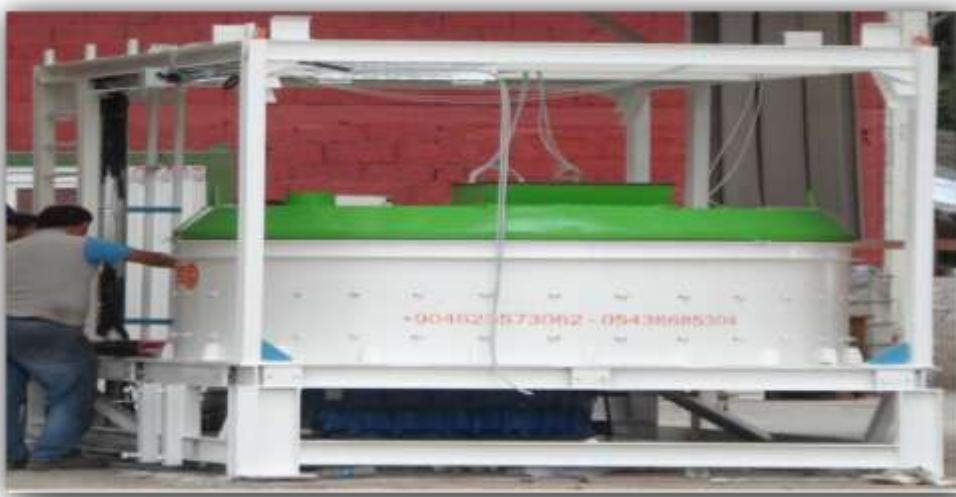
INSTALLATION PLATFORM FOR TWINSHAFT AND PAN TYPE MIXERS. MANUFACTURED USING NPU 120. BESIDES IS A WALKING PLATFORM FOR THE OPERATOR. IS DESIGNED FOR INSTALLATION OF 1 MIXER.
