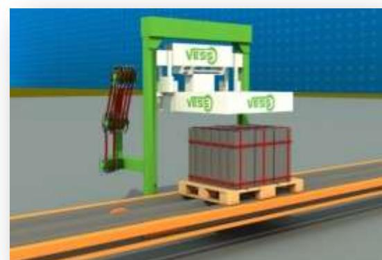
VERTICAL AND HORIZONTAL STRIPING EQUIPMENTS FOR THE PRODUCTS, STACKED ON THE EURO PALLET BY CONCRETE PRODUCT COLLECTING ROBOT. HAS THE FEATURE TO OPERATE FULLY AUTOMATIC.
