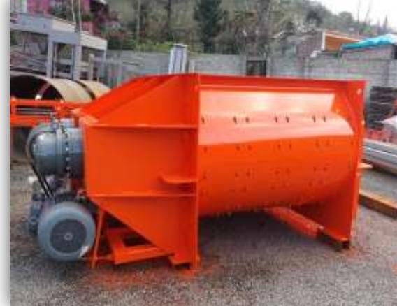
THE MIXER IS PROVIDING HOMOGENEOUS MIXING OF AGGREGATE. MOTOR POWER IS 2 x 45 kw. HANDLE SYSTEM IS AS REPLACEABLE DESIGNED. BY THE PALLETS HANDLE - BY BASE WEAR PLATES AND BY ABRASION SHEET METAL HARDOX / ST 52 - A1 QUALITY MATERIAL IS USED.
