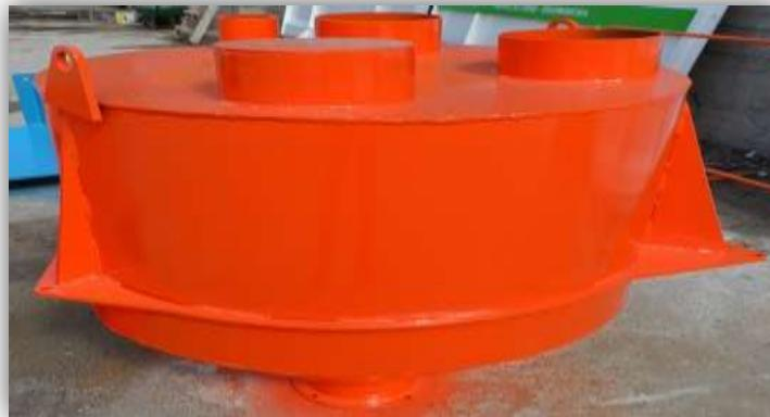
THIS DEVICE IS PROVIDING THE WEIGHING AND SENDING MATERIALS SUCH AS CEMENT – COLOR PIGMENT AND ADDITIVES TO THE MIXER. THE WEIGHING IS PROVIDED WITH 3 PIECES OF 1000 Kg. LOADCELL. WAM BRAND ACTUATOR WITH VALVE AND MICRO SWITCH IS USED. **WATER** ; WILL BE ADDED TO THE MORTAR VIA WEIGHING HOPPER OR DIGITAL WATER METER. THE CAPACITY OF ADDITIVE WEIGHING HOPPER IS 100kg. COLOR PIGMENT WEIGHING HOPPER IS 150kg.
