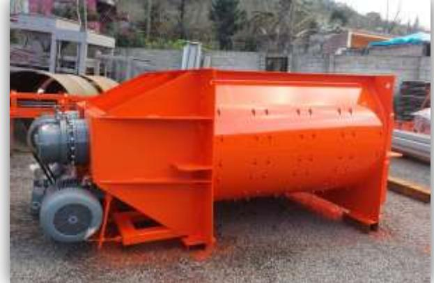
THE MIXER IS PROVIDING HOMOGENEOUS MIXING OF AGGREGATE. MOTOR POWER IS 2 x45 kw. HANDLE SYSTEM IS AS REPLACEABLE DESIGNED. BY THE PALLETS HANDLE - BY BASE WEAR PLATES AND BY ABRASION SHEET METAL HARDOX / ST 52 - A1 QUALITY MATERIAL IS USED.
