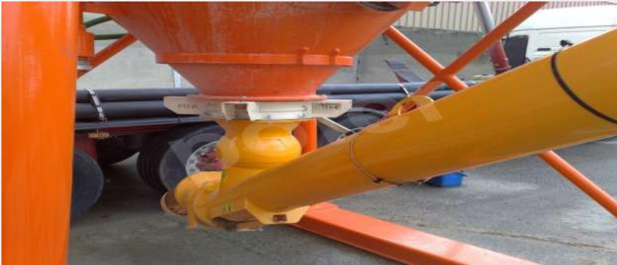
TAKES THE NEEDED CEMENT FOR MORTAR FROM THE SILO TO FEED THE WEIGHING CONVEYOR . WAM BRAND. 8'(Ø219 mm ) MOTOR POWER IS 9,2 Kw. SILO CONNECTION POINT IS MOVABLE.
